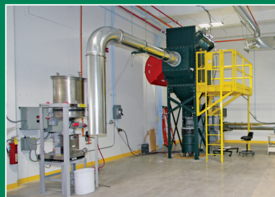
ASHRAE Standard 199 Dust Test Apparatus
